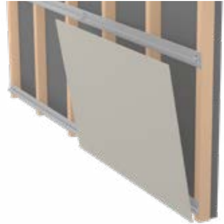
2 Place module, inclination is possible for cabling.
