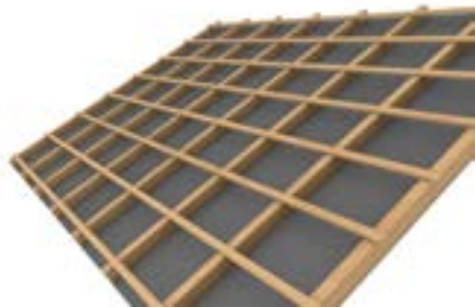
1 Preparing the roof battens
