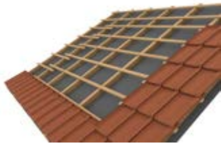
1 Preparing the roof battens
