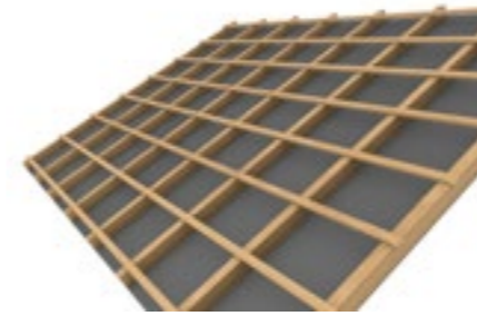
1 Preparing the roof battens
