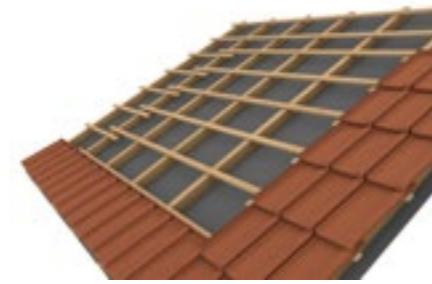
1 Preparing the roof battens
