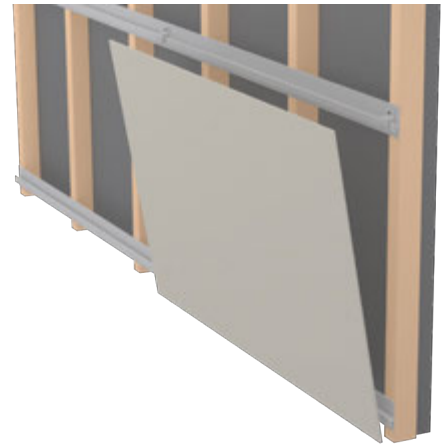
2 Place module, inclination is possible for cabling.
