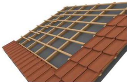
1 Prepare roof battening
