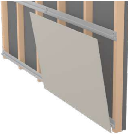
2 Place module, inclination is possible for cabling.
