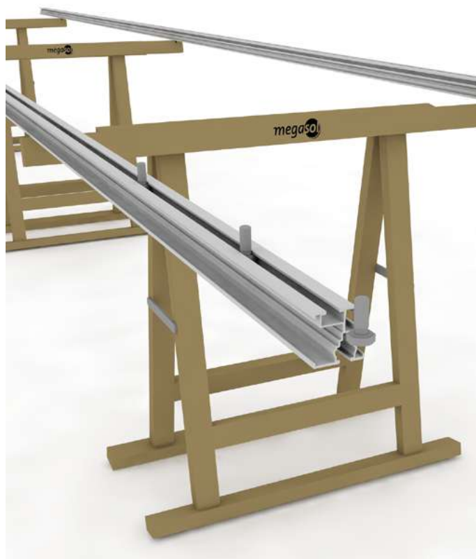
1 Place the LOCKUP rail on Megasol trestles and insert M10x25 hexagon screws into the rail.
