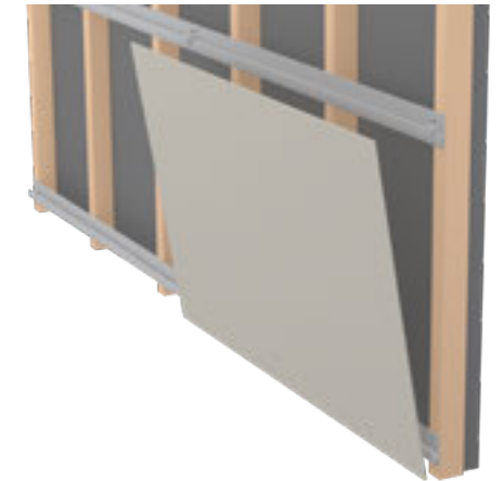
2 Place module, inclination is possible for cabling.
