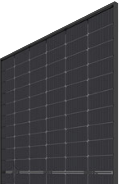
Mono HiR Bifacial M6 HC120 | Full Black Optik Zelltyp: n-type HiR M6 (166 mm) Zellmatrix: 120 Half-cut Zellen Rahmen: U30 schwarz
