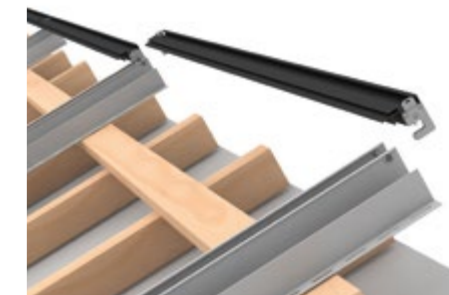
3 The roof ridge profiles are then installed.
