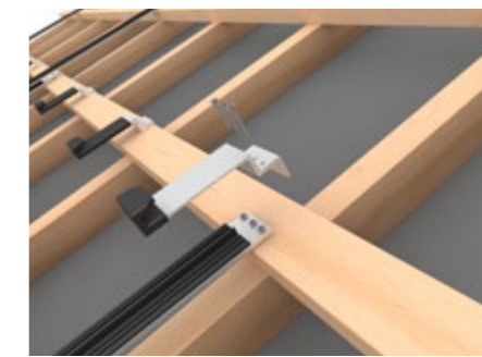
2 The rail hooks are mounted directly on the roof battens.
