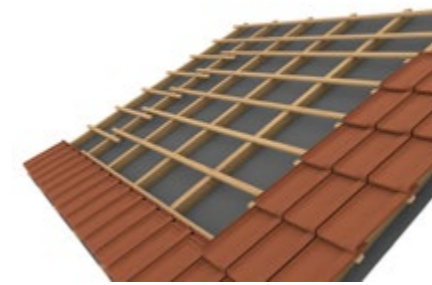
1 Prepare roof battening
