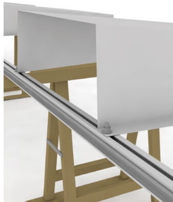
2 Place the Flatport trays upside down on the rails and tighten them with M10 flange nuts.
