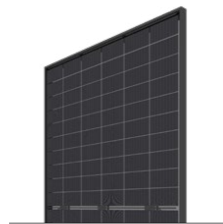
Mono HiR Bifacial HC120 G1 | Full Black optics Cell type: n-type HiR G1 (158.75 mm) Matrix: 120 half-cut cells Frame: U30 black
