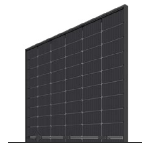
Mono HiR Bifacial M10 HC108 | Full Black optics Cell type: n-type HiR M10 (182 mm) Matrix: 108 half-cut cells Frame: U30 black
