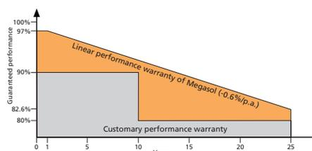
Relative efficiency level in relation to the minimal output (%). At least 97% of the minimum output during the first year. Afterwards, max. 0.6% degradation per annum. At least 91.6% of the minimum output after 10 years. At least 82.6% of the minimum output after 25 years. All data within the measuring tolerances. Warranties according to the respective latest Megasol Warranty Conditions which can be found on [www.megasol.ch/warranty](http://www.megasol.ch/warranty).
